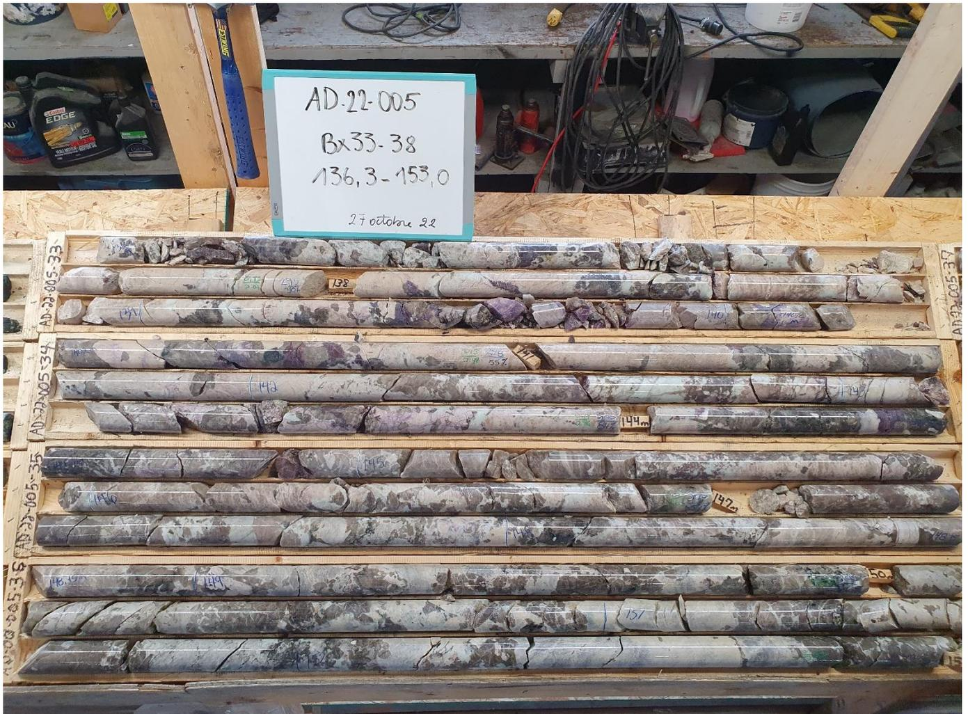
**Figure 3 – Core Samples from hole AD-22-005, Adina**
