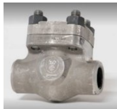
Figure 45. 3D printed drain strainer orifice 3D printed at HII-NNS.
