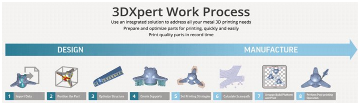
Figure 32: Example of production process planning, illustrated by 3D Systems' 3DXpert software suite
