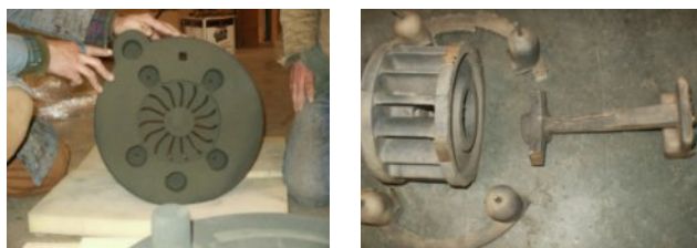
Figure 44. 3D print / sand-casted vacuum rotor (U.S. Navy)
