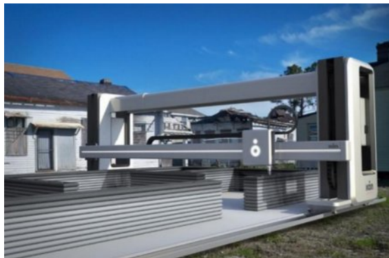
Figure 19. ICON's Vulcan 3D printed construction system. Source: DesignBoom
