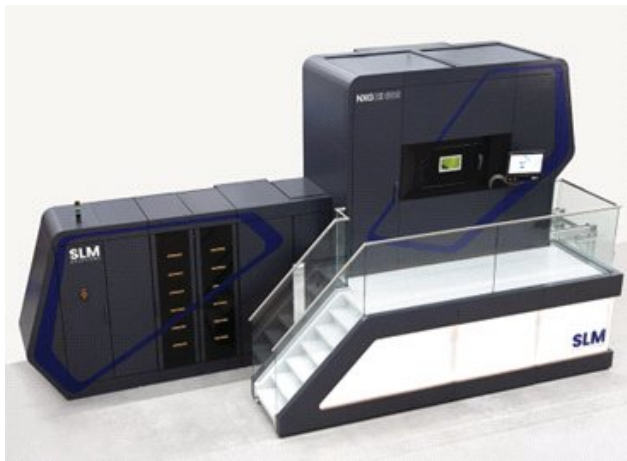
Figure 35. Example of large 12 laser industrial powder bed fusion system from SLM Solutions.
