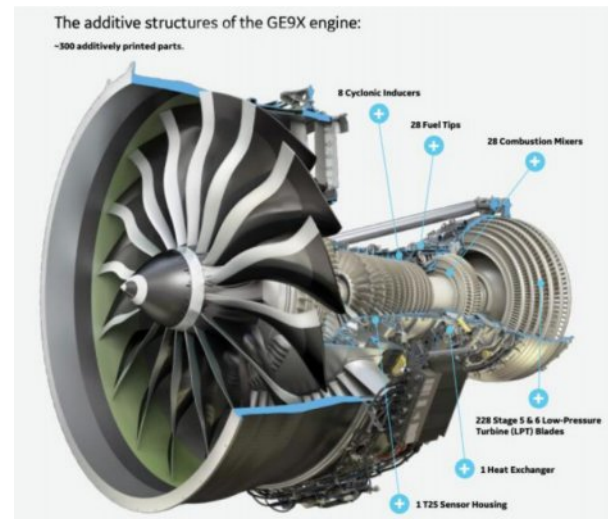
Figure 13. Ranked the world's most powerful engine by Guinness World Records, the GE9X engine uses more than 300 AM parts. (Source: GE Additive)
