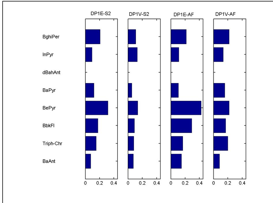
**Figure 9: PAH concentrations (ng/m<sup>3</sup>) measured in the First Deck Park tunnel experiment (before repaving).**
