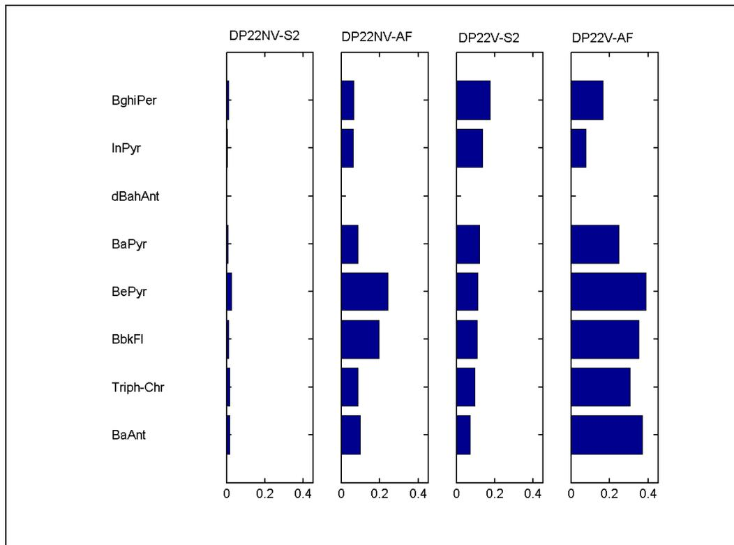
**Figure 11: PAH concentrations (ng/m<sup>3</sup>) measured during the second day of the Second Deck Park tunnel experiment (after repaving).**
