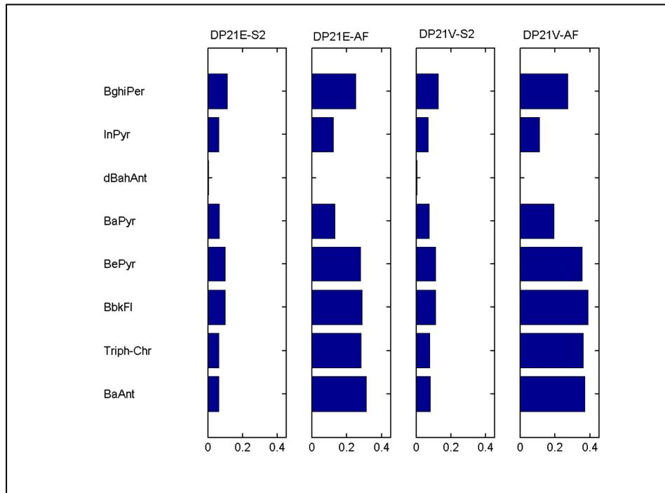
**Figure 10: PAH concentrations (ng/m<sup>3</sup>) measured during the first day of the Second Deck Park tunnel experiment (after repaving).**
