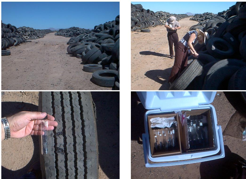
**Figure 3: Tire tread samples collected from the Queen Creek Crumb Rubber Recycling plant.**
